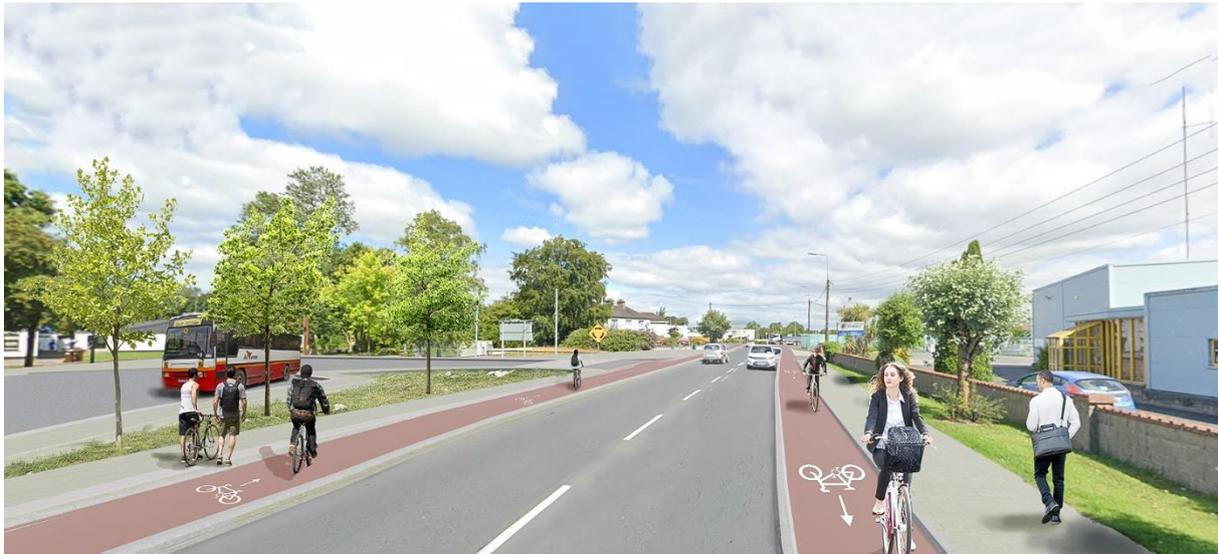
**Figure 6.3: Example of Segregated Cycle Route along R498 outside of Colaiste Mhuire**
