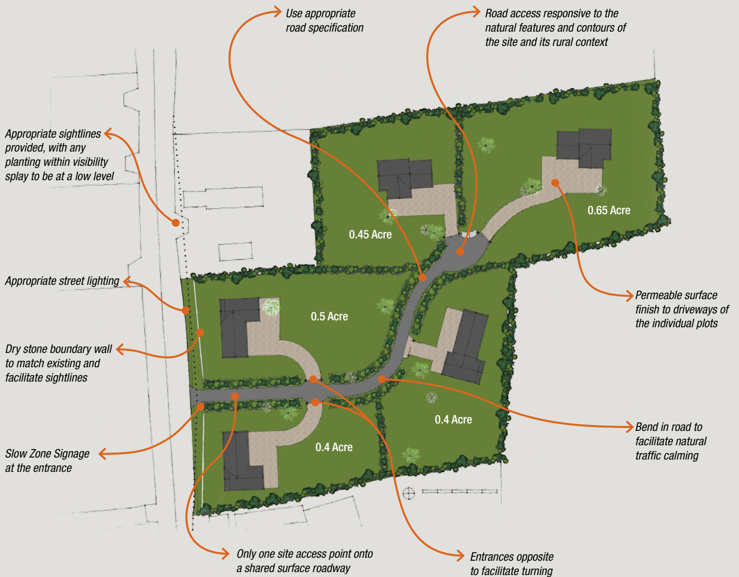
Figure 10: Site strategy highlighting roads infrastructure guidelines
