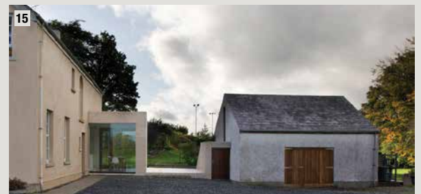
Permeable surfaces (e.g. pea gravel and small scale stone paving) for hard landscaping of driveways and external patios, with use of natural, earthy colours sympathetic to local landscape.
