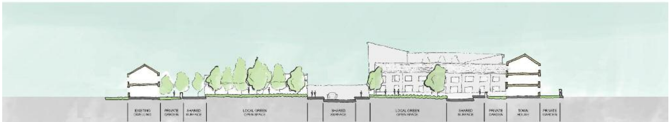
SECTION THROUGH RESIDENTIAL AT MARTYRS' ROAD: Open spaces set on both sides of road can be landscaped to achieve a sense of a coherent single open space.
