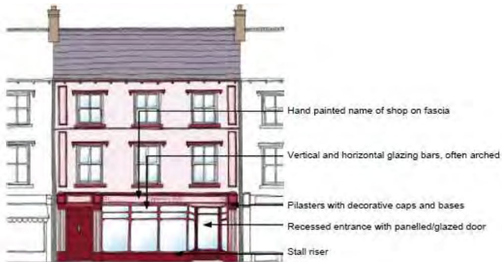
Figure 9.1 – Elements of a Traditional Shop Front
