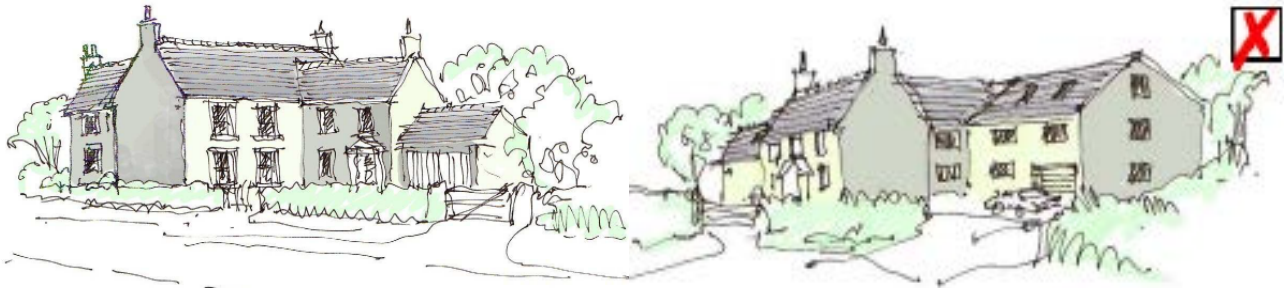
Appropriate extension, subservient to main house and of same materials existing house.
