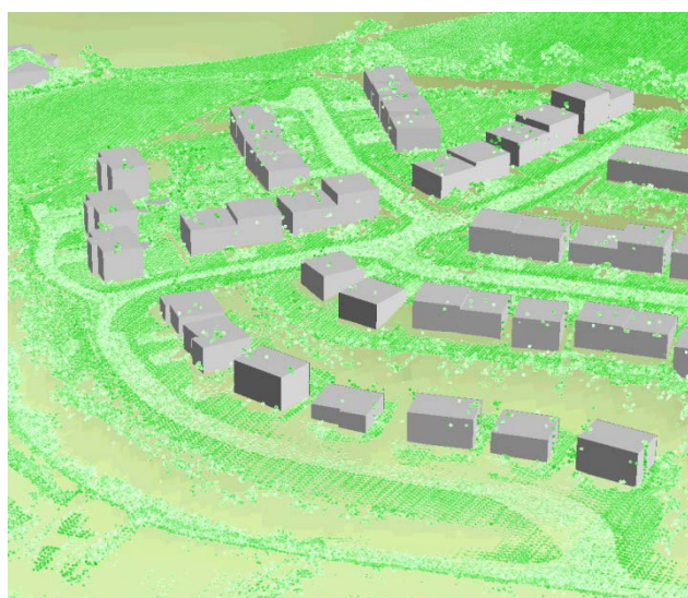
Figure 2: Sample Point Cloud from Aerial LiDAR Survey
