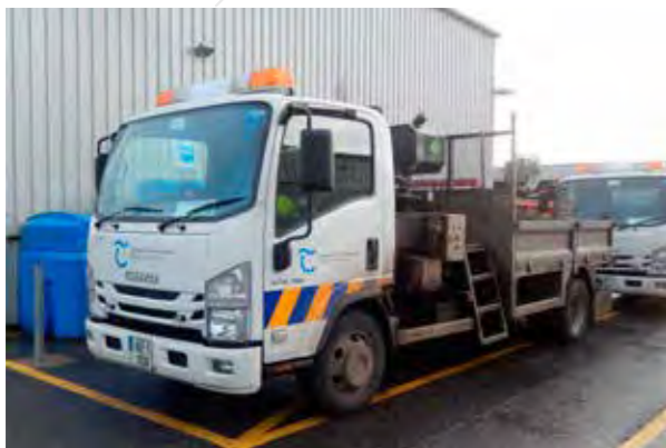
One of 2 New ISUZU 7.5 Tonne Patching Units Purchased in 2016
