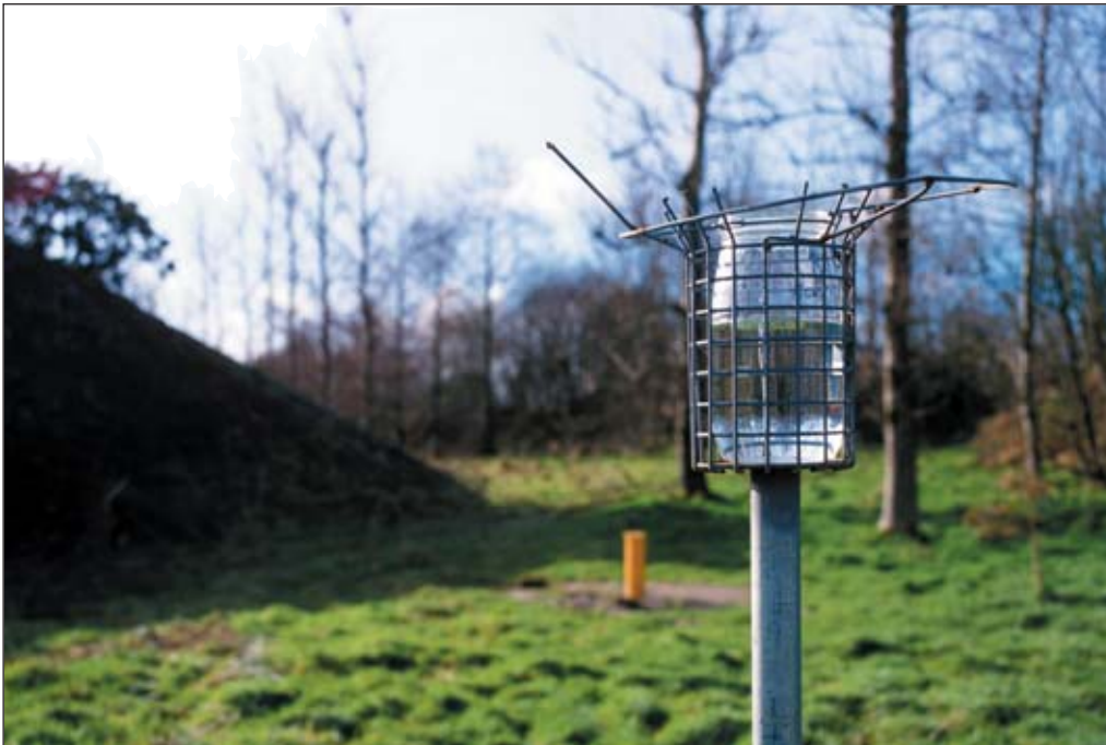
Bergerhoff gauge used to measure the concentration of lead in deposited dust
