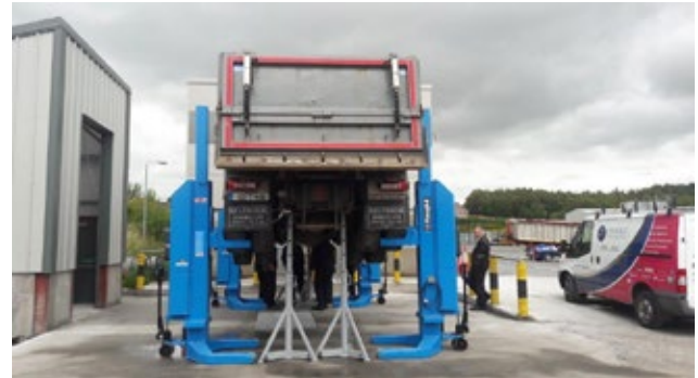
Truck lift system for washing underside of vehicles
